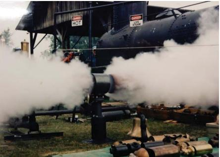
Restoring the whistle is necessary before creating the sculpture. Part of the restoration is to test the whistle with steam and ensure it functions properly or if it is in need of any repairs.
